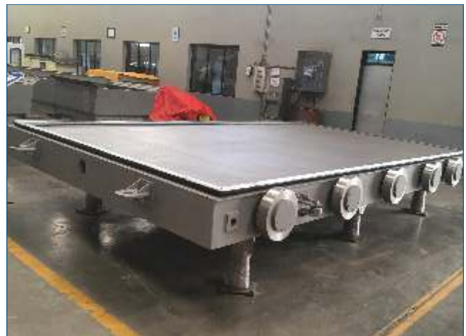
2700 x 6100 mm Stainless Steel Roller Gates for Mississippi Floodwall ORS Pump Station Rehabilitation - Phase III Saint Louis, MO, USA
