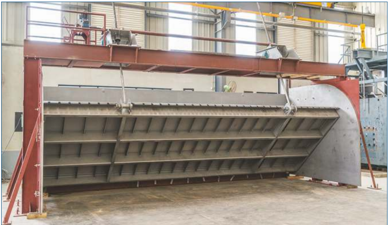
7850 x 2350 mm Stainless Steel Tilting Weir Gate for CWRP C21B, Singapore
