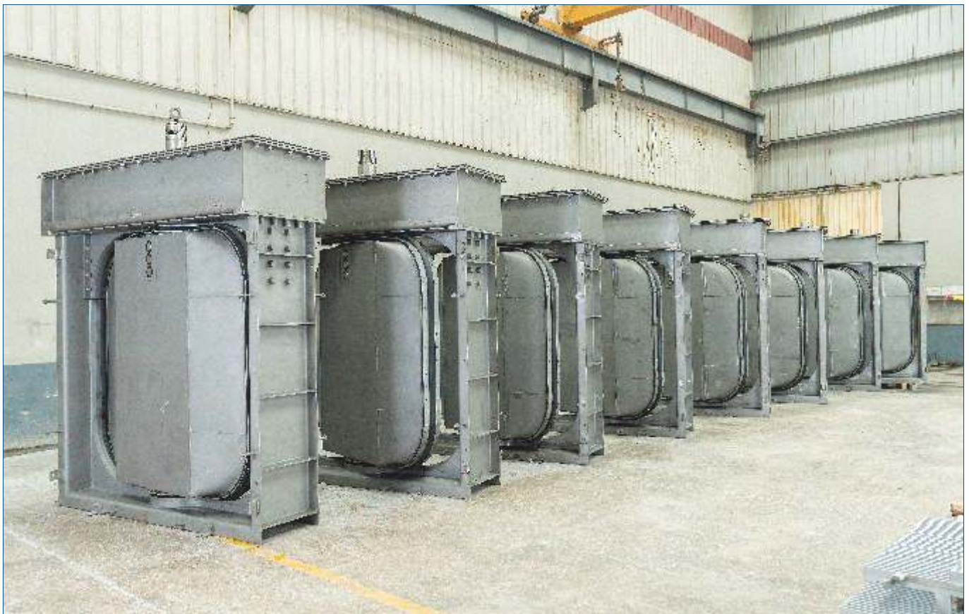
1950 x 1900 mm Super Duplex Stainless Steel Turning Valve for Pulau Tekong, Singapore
