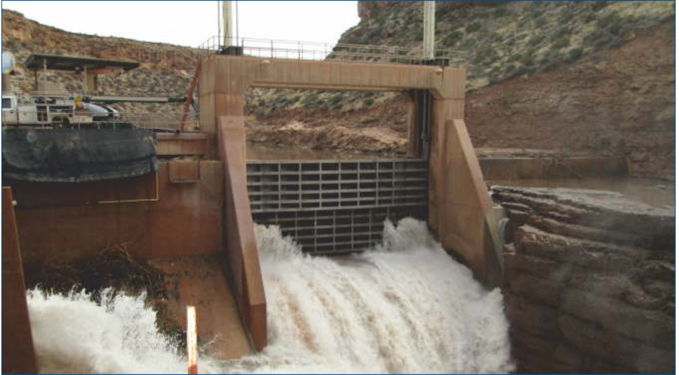
12000 x 6000 mm Stainless Steel Roller Gate for Quail Creek Reservoir, UT, USA Comprising of two 12000 x 3000 mm Gates, Operating Independently to Provide Overflow or Aperture Discharge
