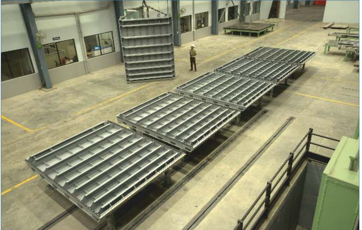
3000 x 3650 mm Structural Steel Bulkhead Gates for Indianford Discharge Capacity Upgrades, Rock County, WI, USA
