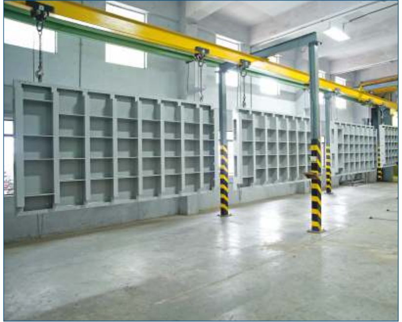
2100 x 3600 mm Structural Steel Stop Logs for Catskill and Delaware Water Treatment Facility, NY, USA
