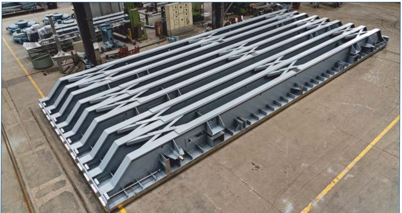
15000 x 6000 mm Structural Steel Bulkhead Gates for San Joaquin River Authority, CA, USA
