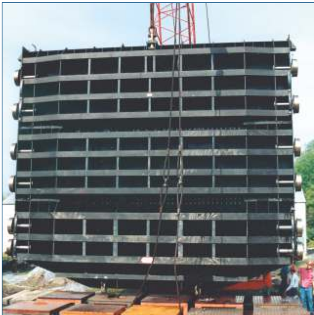
9100 x 8650mm Roller Gate for Idaho Power's Swan Falls, ID, USA
