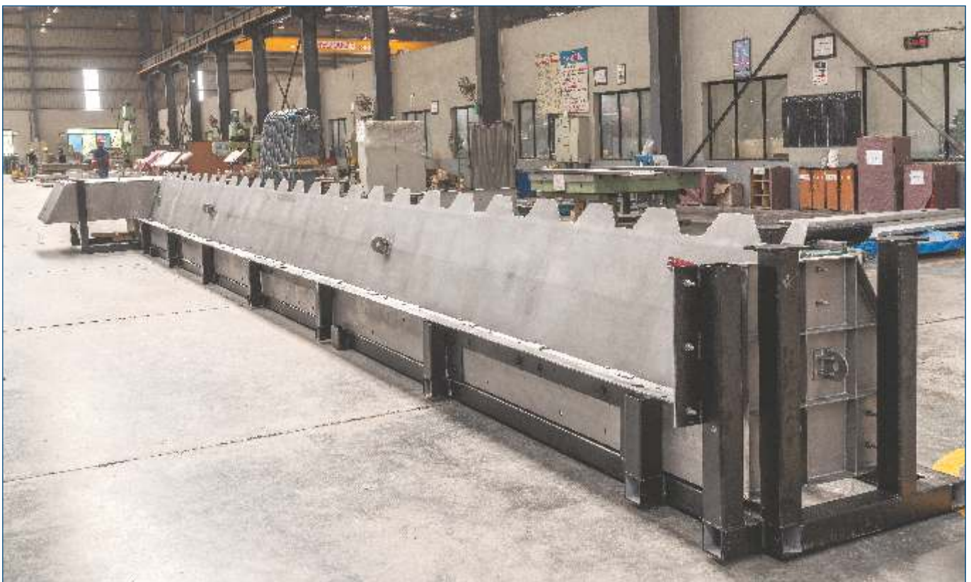
12000 x 600 mm Stainless Steel Bascule Crest Gate for Chocolate Bayou, TX, USA
