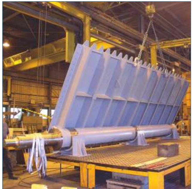
7600 x 3050mm Structural Steel Crest Gate for Newton, NC, USA
