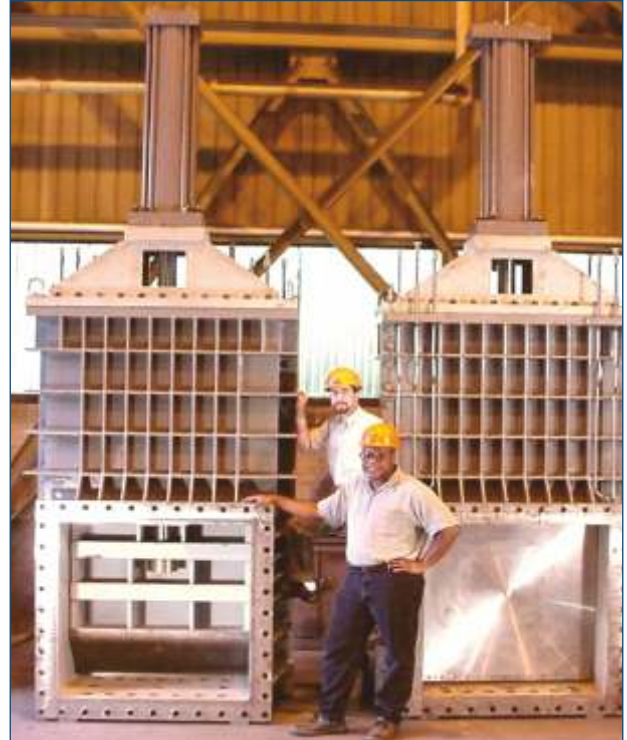
1200 x 1200 mm Stainless Steel Bonneted Gate, Confederated Salish & Kootenai Tribes, Ronan, MT, USA
