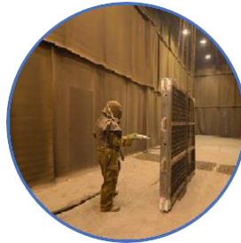
Shot blasting of carbon steel up to 5000 x 4000 x 20000mm
