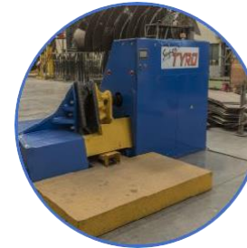
Flight Forming Machine for 5000 mm diameter
