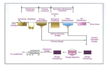
In primary sedimentation tank, about 50% of the suspended solids are settled out & removed as primary sludge by sludge scrapper mechanisms. There are 8 existing primary sedimentation tanks in which tank 4 & 6 were set for refurbishment due to aging of mechanisms.
