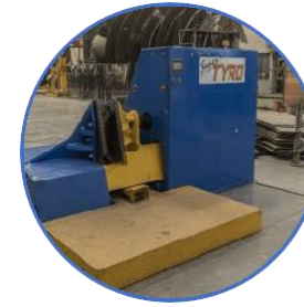
Flight Forming Machine for 5000 mm diameter
