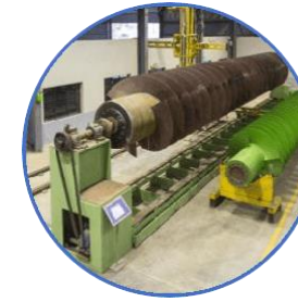
Flight welding machine for 4500 mm diameter x 24,000 mm length
