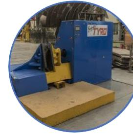
**Flight Forming Machine for 5000 mm diameter**
