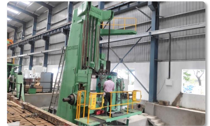
Schies - Horizontal Boring Machine
