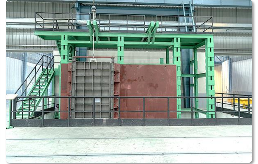
Pic: Stainless Steel Gate 1815 x 4936 mm for project Dalmarnock WWTW Scottish Water, UK.
