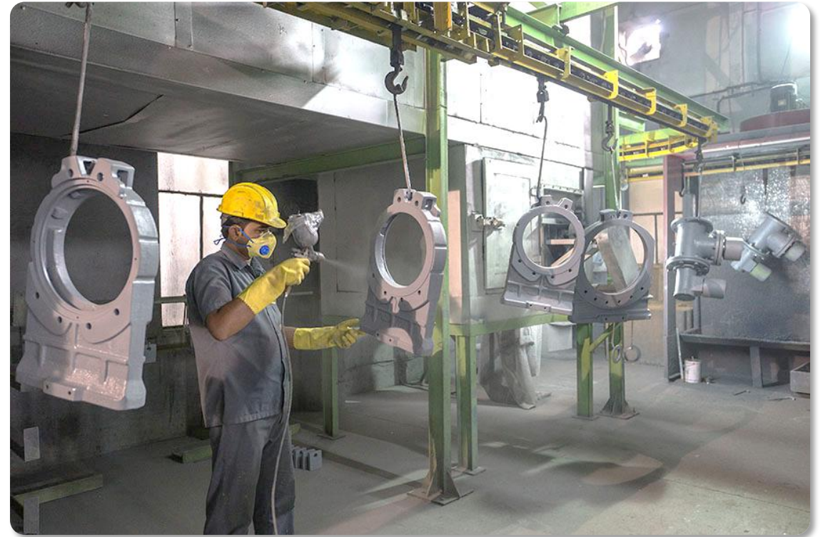
Valve Paint Shop
