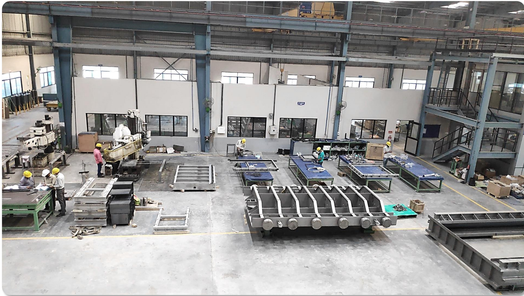
Stainless Steel Gate Assembly Shop
