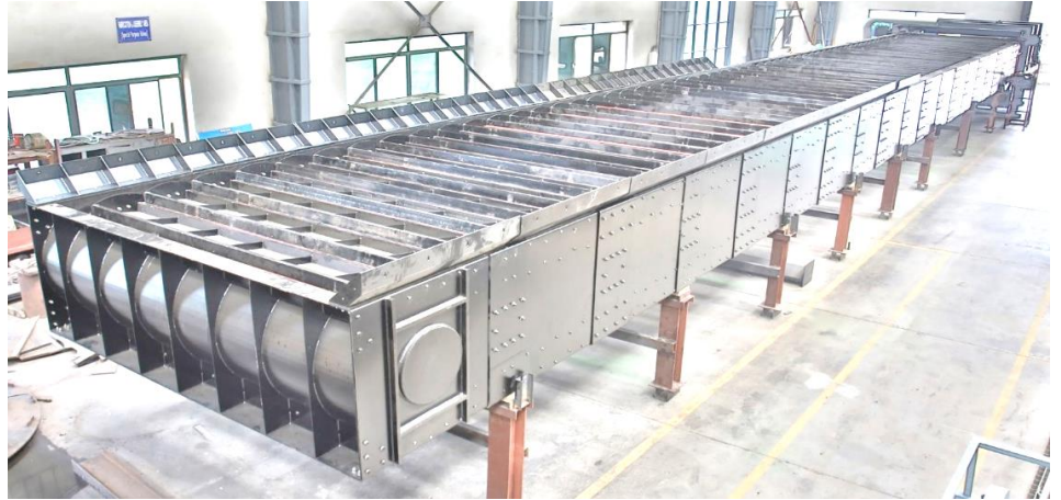
Complete Screen of over 31.54 m length in operational testing at Jash for Vizag Steel Plant, Visakhapatnam, India
