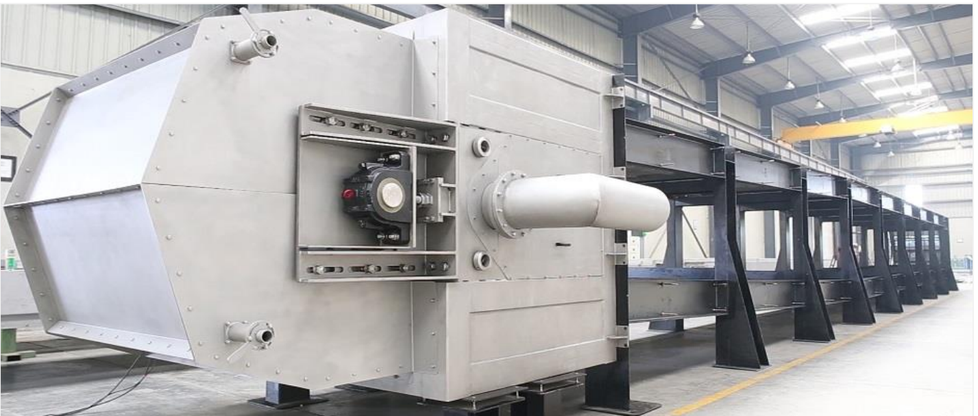
Complete Screen of over 31 m length in operational testing at Jash for RSPL Sea Water Intake, Dwarka, Gujrat, India.
