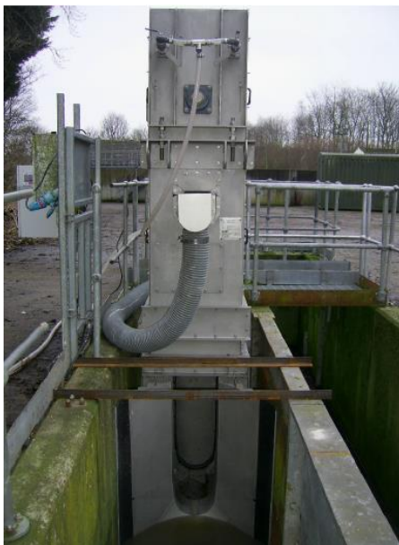
Jash-Mahr Band Screen during testing at NSEF, UK
