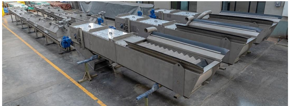
Screens & conveyors with washer compactor for Las Pinas Project, Philippines
