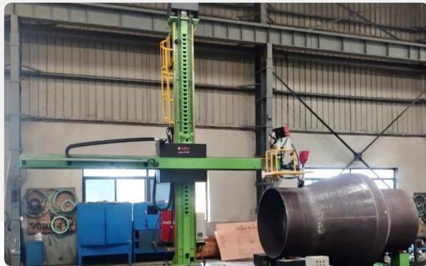
SAW Welding on Diameter upto 5000 mm
