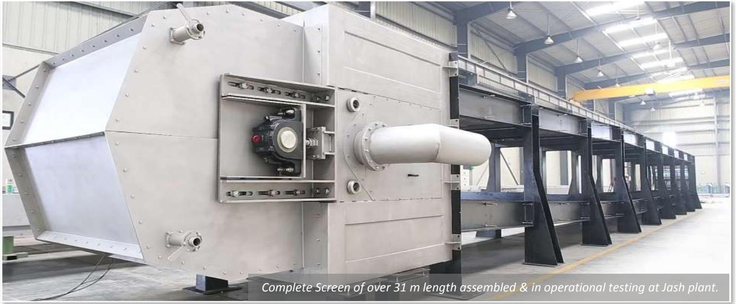
*Complete Screen of over 31 m length assembled & in operational testing at Jash plant.*
