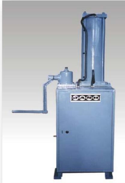
Pneumatically operated lift mechanism is provided where very fast opening and closing is desired or where fail safe condition is required.
