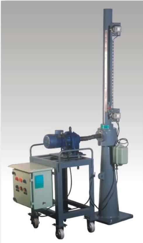
Portable electric operator is provided for faster opening of manually operated gates. A common portable operator can be used for operation of a number of gates of different sizes located near each other.
