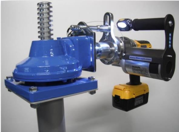
Portable battery driven actuators are provided to operate the gates in event of power failure for electric operated gates.
