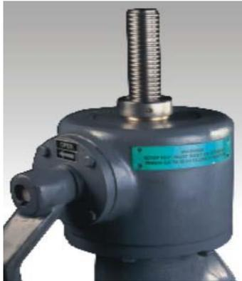
Safety stop nut is provided on threaded rising stems of manually operated gates to prevent chances of over closing of gate and thus to avoid chances of damage to wedge blocks, stem and the operating platform.
