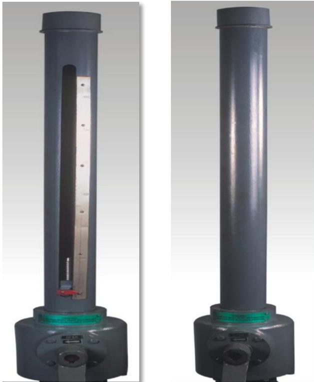
**Cause – c** : A stem that looks well lubricated may still be causing some trouble if the grease is contaminated with rust particles. This happens when stem is covered by a steel or galvanized steel pipe cover. Rusting takes place within the pipe cover and rust particles drop into the grease.
