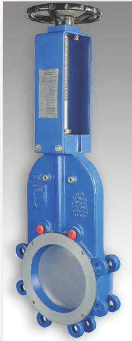
The MONO-A version Knife gate valves are bonneted, full Lug, gland less valve in Ductile Iron construction complying with AWWA C 520-10 standard. Full lug design enable end of line mounting without the need of additional flange. Mono-A version is having a single piece design up to DN 600 and split body design for higher sized valves.
