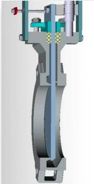
Knife gate valves were developed for isolation of pulp in paper industry where water contains large amount of solids in form of fibrous pulp. The gate of this valve was given a narrow edge at its bottom to enable it cut through settled pulp and achieve full closure of valve.
