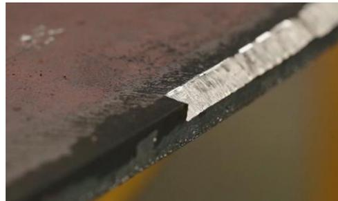
Bevelled and unbevelled surface
