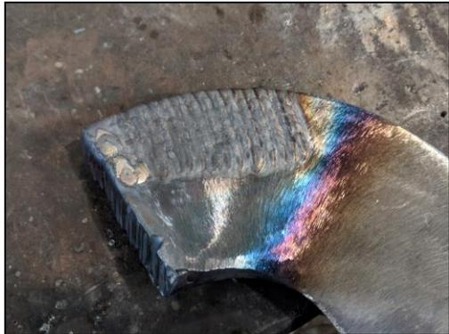
Cobalt Base continues cast hard facing rod for TIG and oxy-acetylene welding. Very good resistance to metal-metal wear, cavitation and corrosion as well as heat up to 900° C. Excellent gliding characteristics, good to polish, non-magnetic. Machinable with tungsten carbide tools or by grinding. Hardness: 43 HRC
