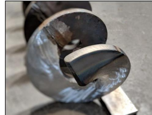
Nickel based hard surfacing alloy, which can be deposited using super flame spraying torch over the surface to be hardened.
