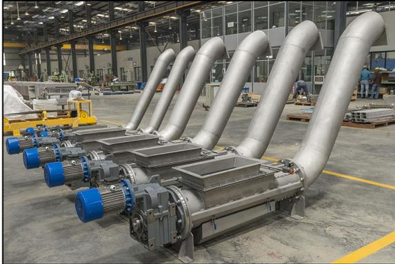
Screw compactor are suitable for washing and compacting the floating waste coming out of the screens and travelling through a belt or screw conveyor in case of multiple screens or directly from the screen in case of single screen installed in municipal waste water pumping station or treatment plant. The Screening wash compactor shall remove the organic material by washing and compaction thus reducing the volume and weight by 40%.
