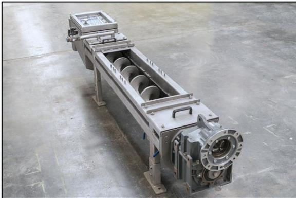
Shaftless Screw or Spiral Conveyor is an alternative concept to the traditional shafted screw conveyor. Material is conveyed by an extra heavy duty shaftless screw that slides on a low-friction, wear-resistant liner inside the conveyor trough housing. Shaftless spiral conveyors are successfully used to transport jamming, bridge forming and sticky materials. JASH shaftless spiral conveyors can be furnished in a wide variety of materials to resist corrosion, abrasion and exothermic conditions.
