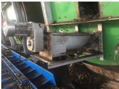
Equipment: Shaftless Spiral conveyor
