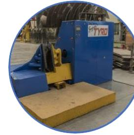
**Flight Forming Machine for 5000 mm diameter**
