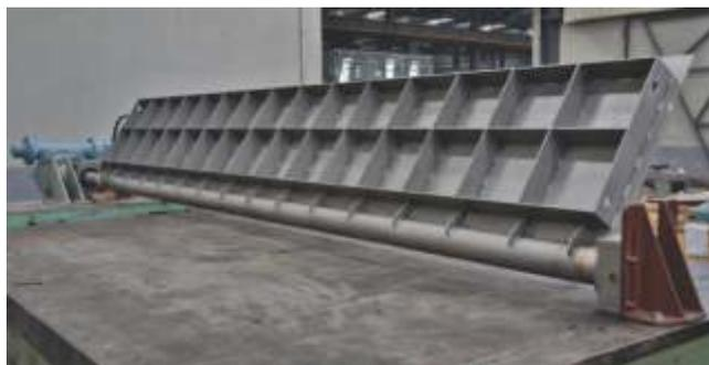
7. Developed & manufactured Vane Gates and butterfly gates for Enviro Control Surat & Rodney Hunt USA. The company is now geared to develop complicated products to suit specific clients requirement.
