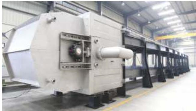
5. Developed & manufactured special seawater intake Travelling band screens for RSPL SODA ASH Package Project at Jamnagar, Gujrat. The length of screen is approx. 25 meters and the width of screen is 1.5 meters and with 2 mm perforations it is the biggest screen in India for such application.
